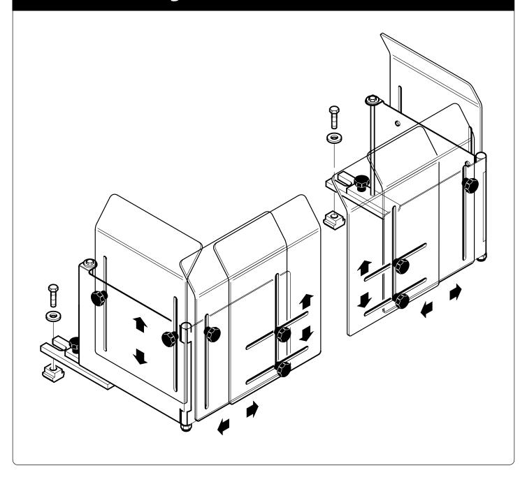
Site one half of the guard onto the machine table in the approximate working zone.
