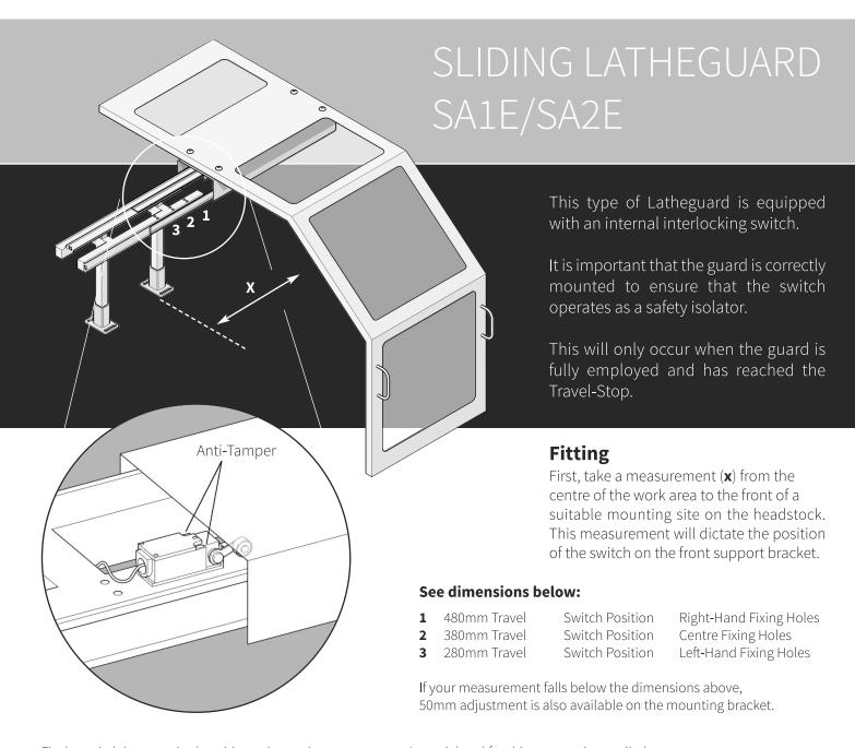
Fix the switch into required position using anti-tamper screws. A special tool for this purpose is supplied.
